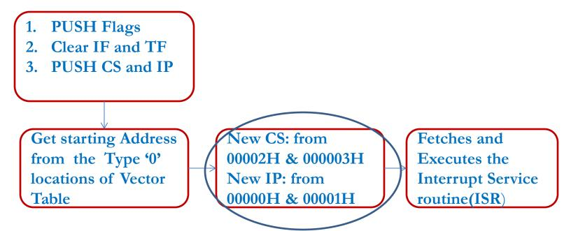
➢ After loading the starting address of the procedure which is written for Interrupt into CS & IP , then 8086 fetches and executes the first instruction of the ISR.
