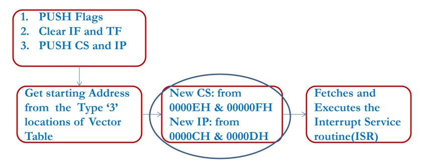
**Type '4' Interrupt** Type '4' Interrupt / Overflow Interrupt When this Overflow Interrupt happens ?
